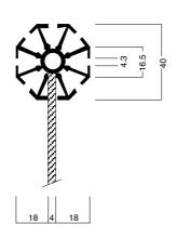
Specification of pole, beam, joint
